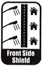
GCJ Type 2 Light Distribution with FSS
