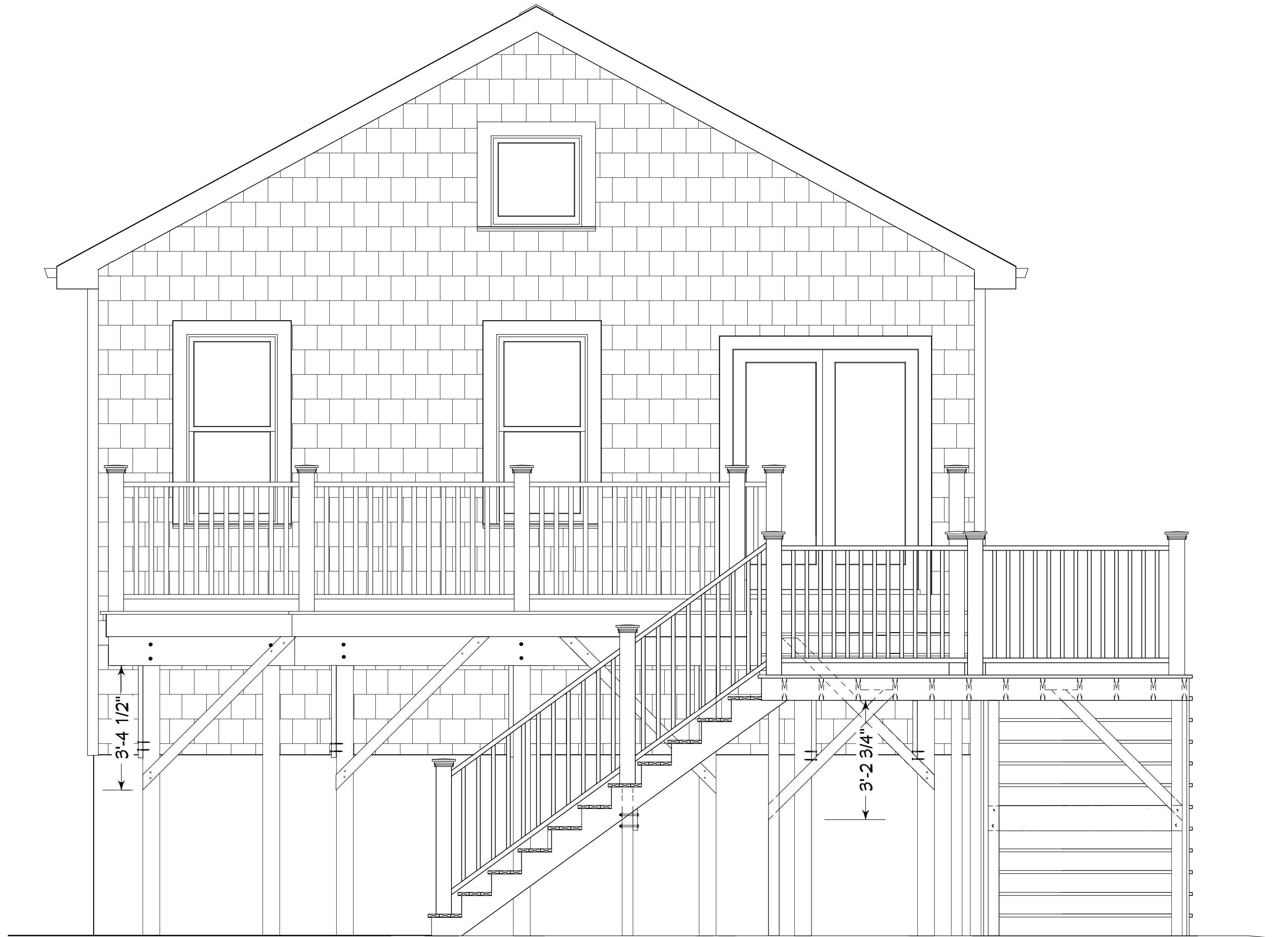
REAR ELEVATION SCALE 1/2" = 1'
