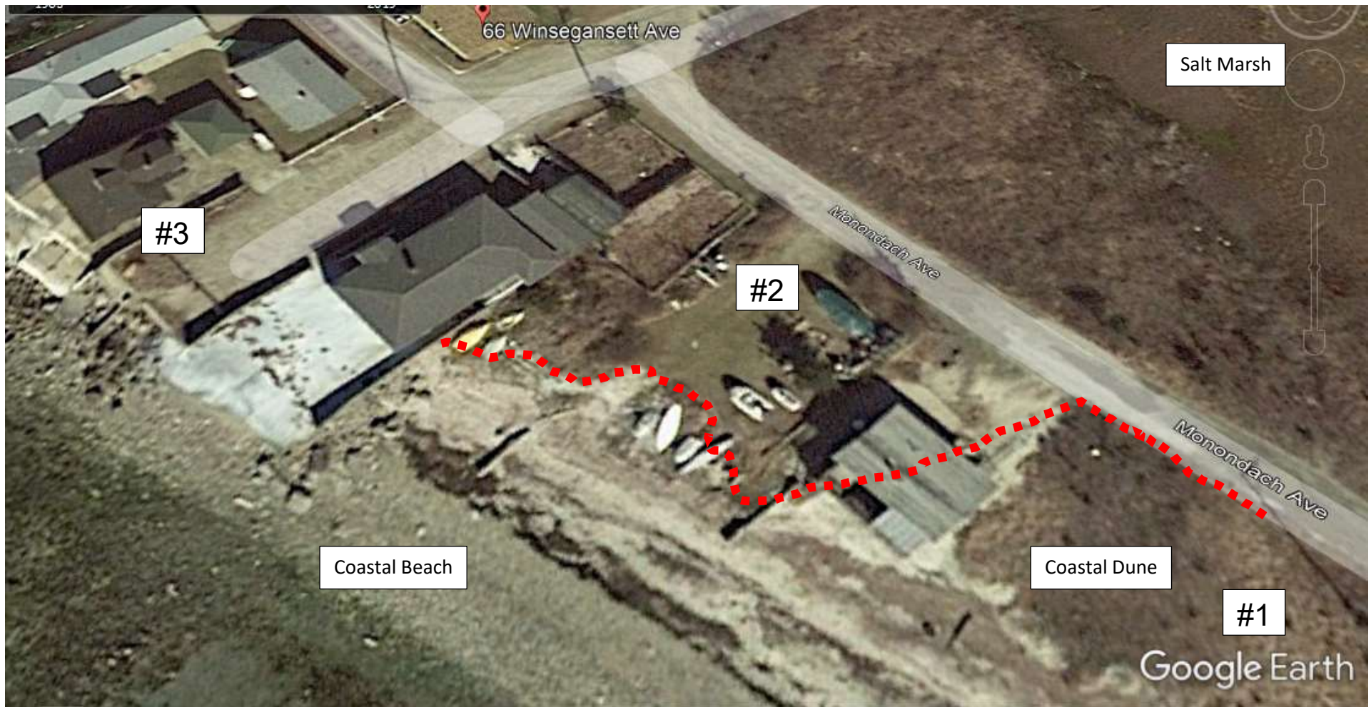
Figure 3a. The landward limit of the Coastal Dune is approximated with the use of aerial imagery and site observations. Sediment samples were taken from a foot below the surface and compared to confirm the presence of glacial material at sites #2 and #3 (see Figure 3b). Windblown sand accumulation was sampled at site #1.
