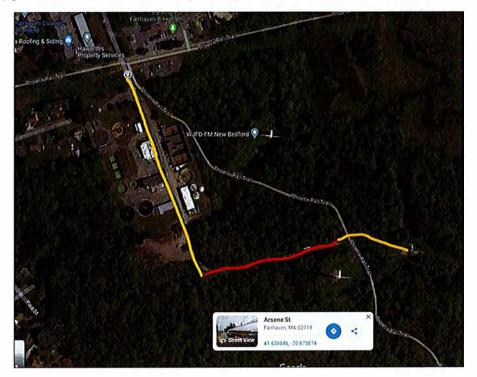
The fiber cable that we would like to place will improve Eversource communications in this area of Fairhaven. Our present system is on Microwave and fog can slow that system. Having good information about how our equipment is working makes everyone safer, improves response times, and keeps the power on. Using a fiber cable provides a consistent path for Eversource communications.
