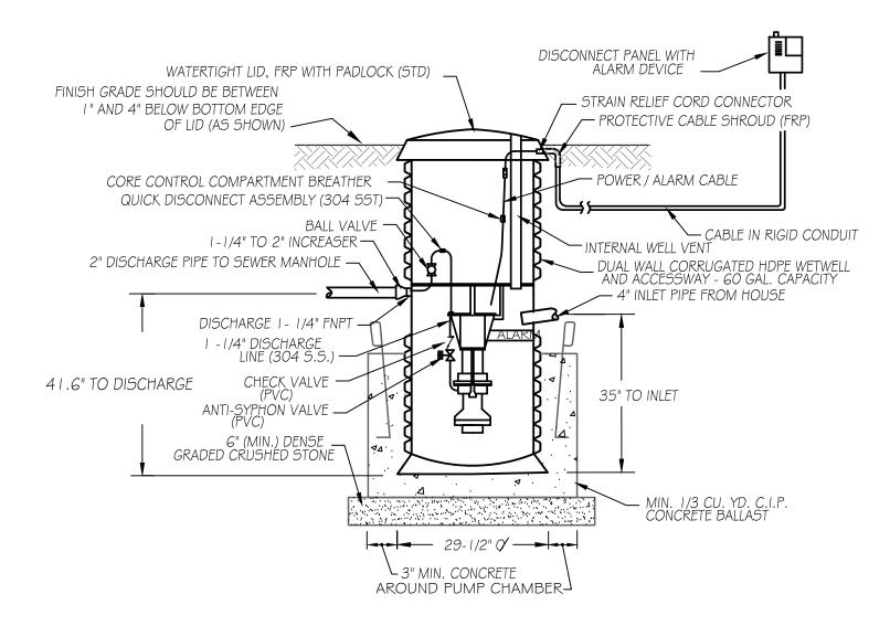
TYPICAL GRINDER PUMP DETAIL (NOT TO SCALE) USE ENVIRONMENT ONE MODEL No. DHO7 I
