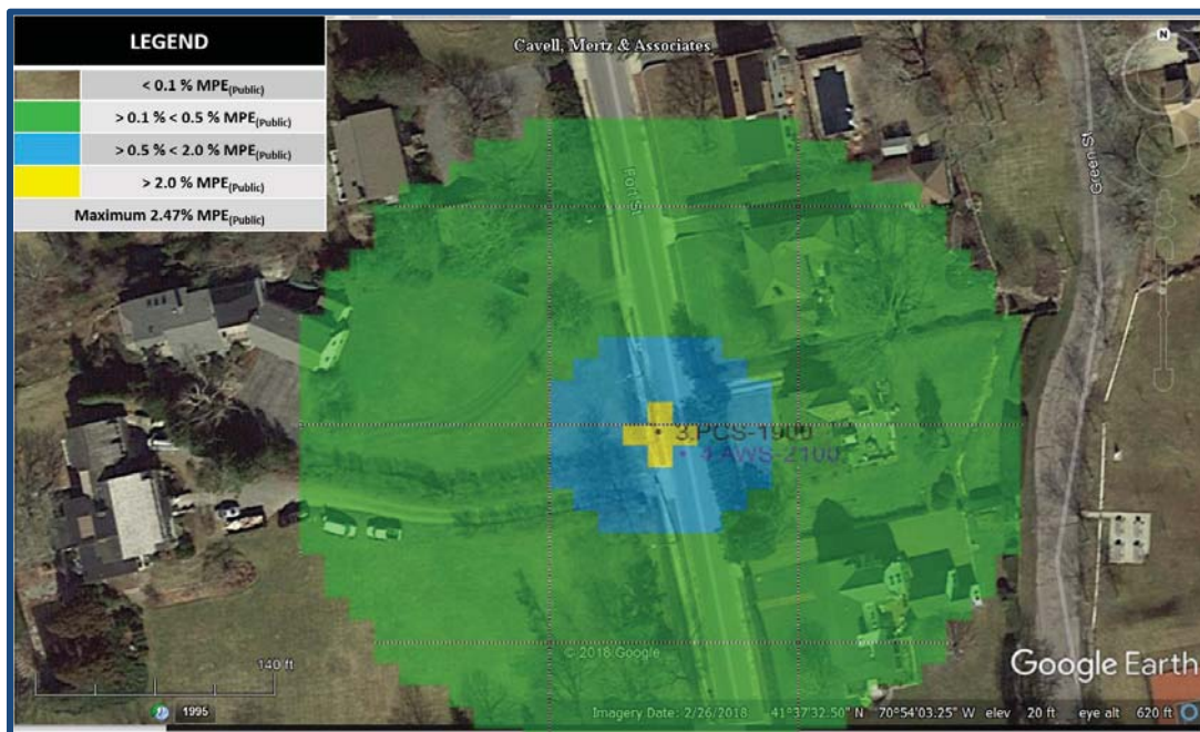
Figure 4: Theoretical Cumulative %MPE (Public) for Ground Locations Utility Pole at 6 Fort Street, Fairhaven, MA (Calculations superimposed over picture courtesy Google Earth ©2019 )
