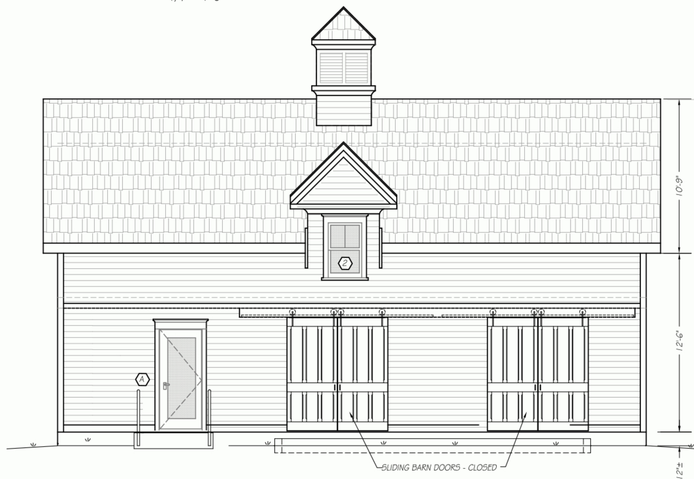
FRONT ELEVATION - DOORS CLOSED 1/4" = 1'-0"
